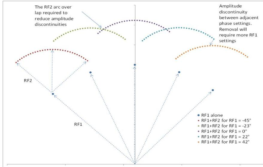
As the phase range and amplitude of RF1 is the same as RF2, the resultant minimum phase step is reduced from 2.8° to 1.4°. To remove any amplitude discontinuities the number of RF1 settings will need to be increased, as shown in **Figure 9**.
