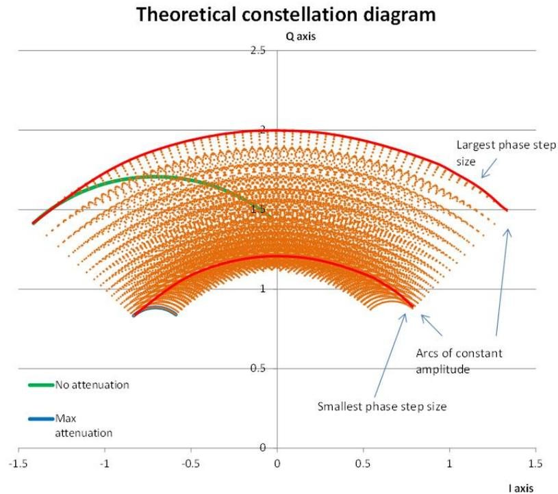
Note that the RF2 arcs remain vertical for all RF1 phase angles. This means that care must be taken to align RF2 arcs, especially at each end of the RF1 phase range. A theoretical algorithm has been determined to align the RF2 curves in order to achieve monotonic phase control, but the PE46120 design contains unavoidable random differential non-monotonicity at certain steps. The overlap factor can be used to compensate for any non-monotonicity.
