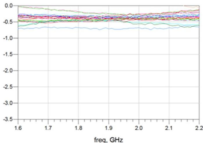
Figure 26 • *Insertion Loss Delta Between Adjacent Phase States (dB, MSB Removed)*
