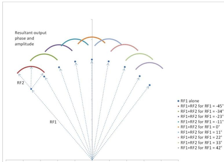
With the RF2 DSA set to 7 dB, the resultant RF2 vector is 0.44. This means the total insertion loss is increased by approximately 2.2 dB, but the resultant output phase resolution is 0.84°.
