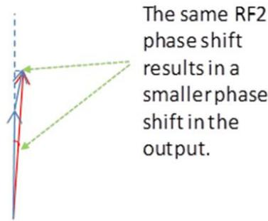
This methodology for obtaining finer resolution can be continued by adding an external attenuator to the RF2 path. With an even smaller signal coming from RF2, the resultant phase shifter signal will tend toward the RF1 signal level, with changes in the RF2 phase setting resulting in even finer phase shifter resolution.
