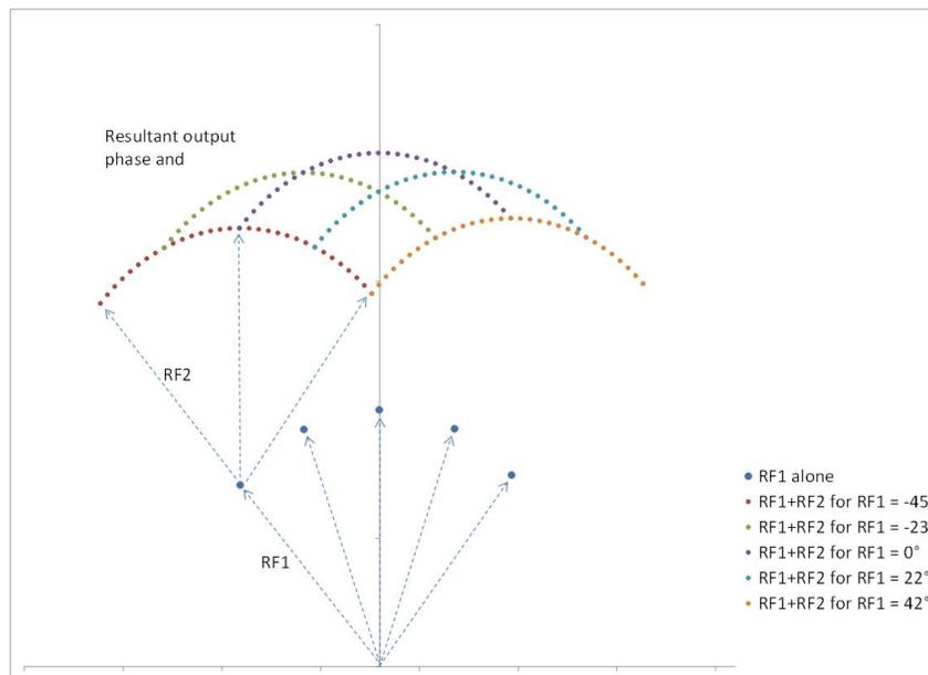
An overlap in the RF2 arcs is necessary to reduce the amplitude variation across the full  $\pm 45^\circ$  range.
