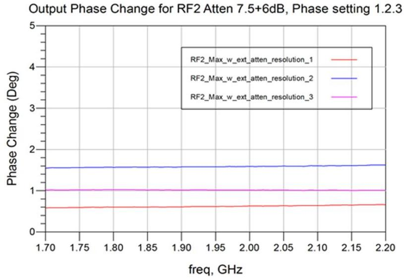
The following are measured results using a 90° hybrid coupler, external 6 dB attenuator and internal attenuator set to 7 dB.
