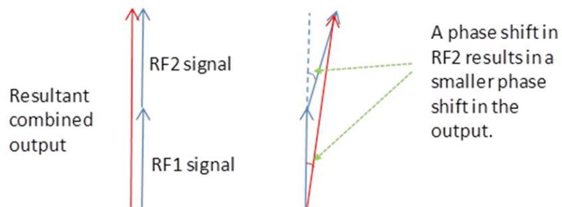
Using the internal DSA in RF2 arm to set 7 dB, any phase step in the RF2 phase shifter will result in a much smaller phase change in the output. The penalty is the reduced level of the signal from the RF2 arm, resulting in an increased insertion loss for the whole phase shifter. This is shown in **Figure 4** as a shorter resultant signal vector. The 7 dB DSA setting and 2.8° RF2 phase resolution results in an output phase step resolution of 0.8°.
