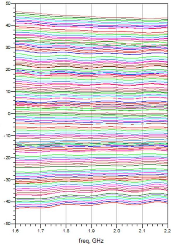
This result is measured across the full phase shift range of  $\pm 45^\circ$  using 5 discrete RF1 phase settings with 24 RF2 phase settings for each RF1 phase setting.
