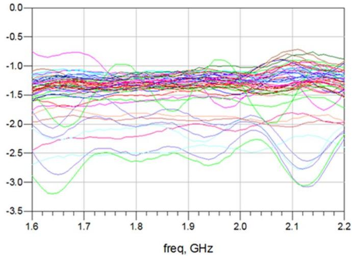
**Figure 17 • Insertion Loss Delta Between Adjacent Phase States (dB)**
