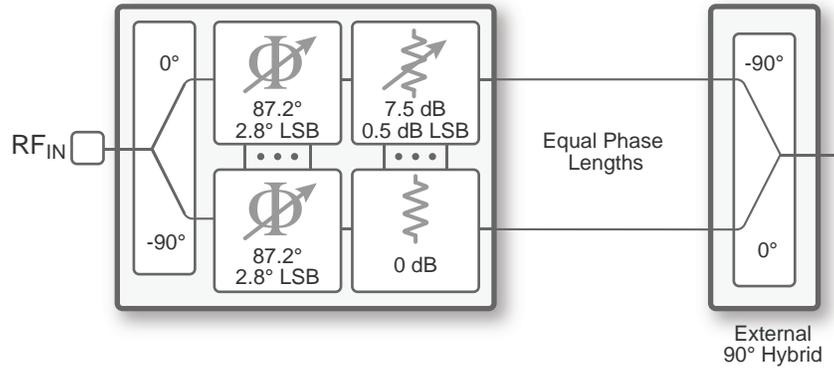
The following are the results of ADS analysis of phase resolution using measured MPAC s-parameters and an ideal ADS 90° combiner model. Figure 14 shows a phase resolution between 1.2° and 1.8°.
