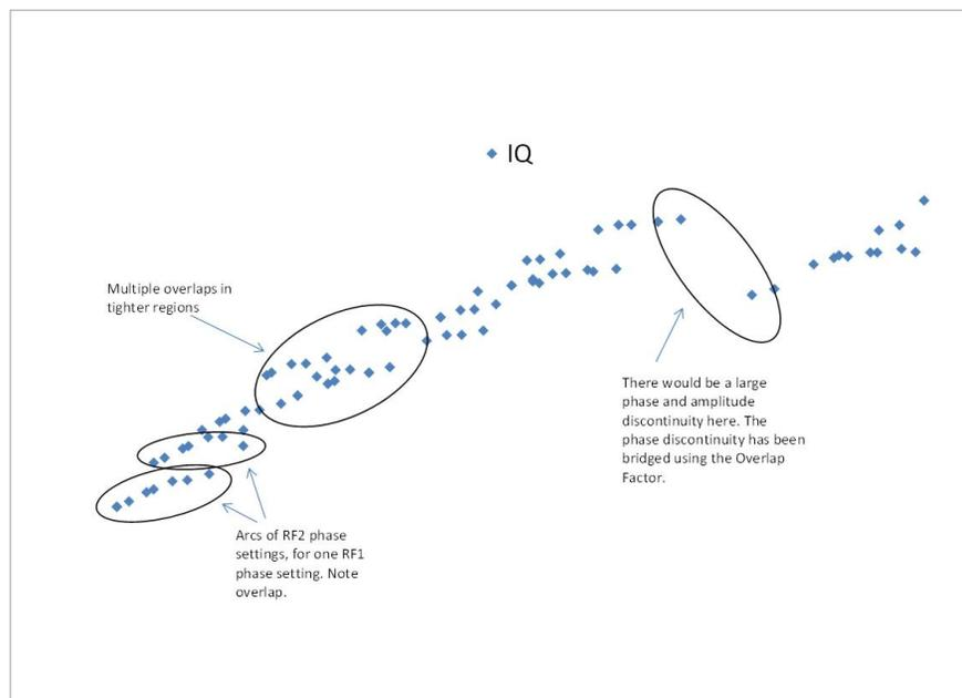
The resulting data shows the non-monotonic behavior, but the gaps have been bridged by use of the Overlap factor. The Overlap factor can be tuned to minimize the number of measurements while bridging the gaps.
