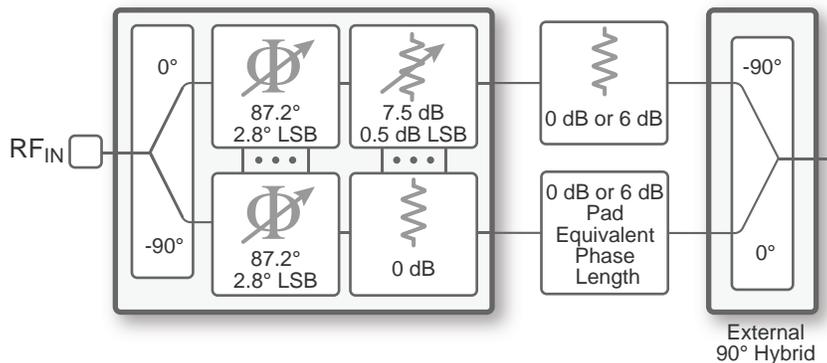
The following are results of ADS analysis of phase resolution using measured MPAC s-parameters and an ideal ADS 90° combiner and 6 dB attenuator model with a phase resolution between 0.4° and 0.6°.
