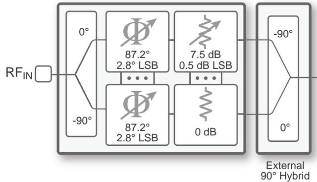
With the RF path attenuator set to 0 dB, and with the phase length in each arm identical such that the signals combine correctly, any phase step in either of the RF1 or RF2 path phase shifter will result in a total signal phase shift of about half the step size of each individual RF path, or about  $1.4^\circ$  in this case, thereby increasing the phase shifter resolution.
