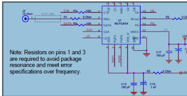
These resistors were originally placed to remove a resonance between the RF<sub>IN</sub> pin and the connection to the adjacent pins. This resonance caused degradation in the PE4304 DSA performance at higher frequencies. The PE4314 does not have this degradation. For the PE4314 it is preferable to remove the resistors or reduce the values such that the PE4314 logic threshold levels are met.
