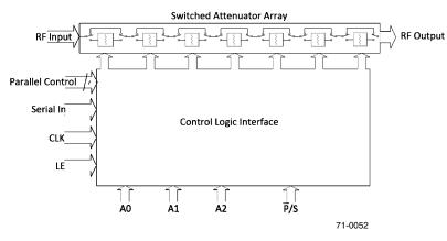
UltraCMOS<sup>®</sup> RF Digital Step Attenuator, 7-bit, 31.75 dB 50 MHz – 8 GHz
