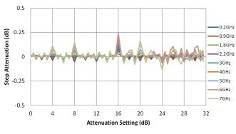
Figure 10. 0.5 dB Step Attenuation vs. Frequency\*
