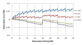
Figure 27. Attenuation Error @ 3000 MHz vs. Temperature
