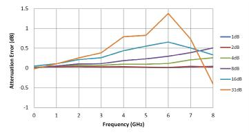
Figure 17. 1 dB Attenuation Error vs. Frequency
