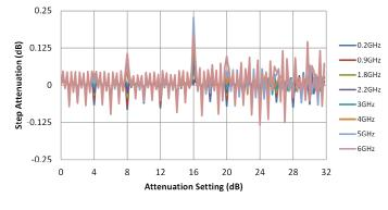
\* Monotonicity is held so long as step-attenuation does not cross below -0.25 dB
