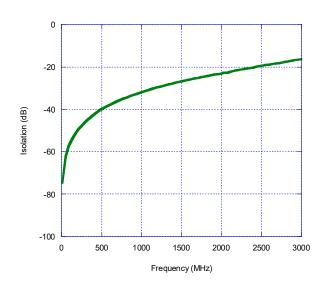
Figure 9. Isolation – RFC to RF2
