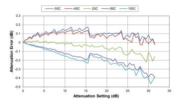
Figure 22. Attenuation Error @ 2.2 GHz vs Temperature
