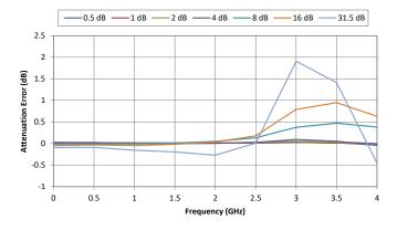
Figure 14. Attenuation Error vs Attenuation Setting
