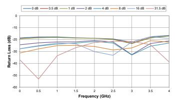
Figure 12. Output Return Loss vs Temperature
