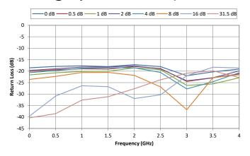
Figure 10. Input Return Loss vs Temperature
