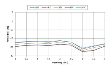
Figure 11. Output Return Loss vs Frequency @ Major Attenuation Steps
