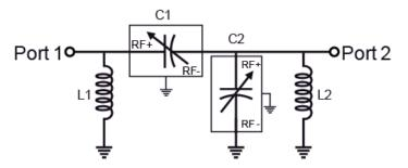
Figure 18. Recommended Layout of Multiple DTCs
