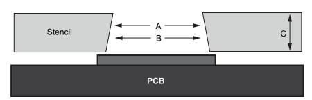
Figure 5 • Solder Stencil Profile (Side View)
