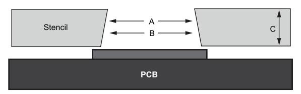
Stencil apertures should be tapered to produce more uniform release of solder paste.
