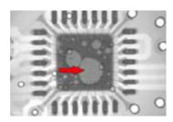
Figure 10 shows the optical image of a cracked solder joint.
