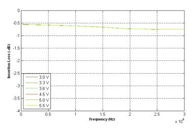
Figure 7. Insertion Loss: RFC-RF @ 3.3 V
