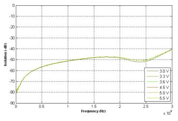
Figure 9. Isolation: RFC-RF @ 3.3 V
