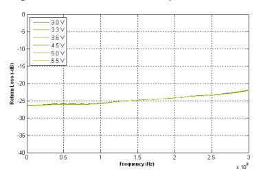
Figure 11. Return Loss at active port @ 3.3 V
