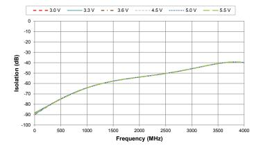
Figure 9. Isolation: RFC-RF @ 3.3V
