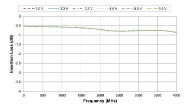
Figure 7. Insertion Loss: RFC-RF @ 3.3V
