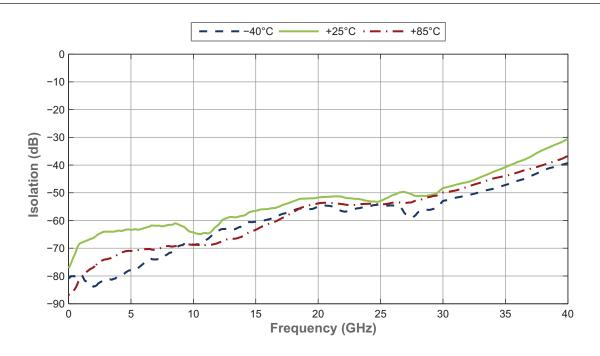
Figure 12 • Isolation vs V1/V2 (RFC-RFX)
