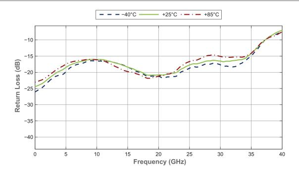
Figure 8 • Active Port Return Loss vs V1/V2
