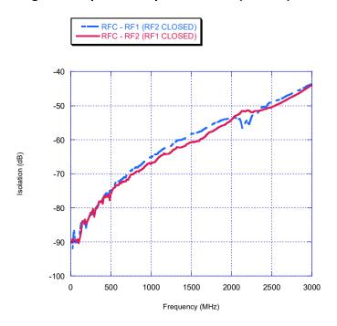
Figure 8. Input to Output Isolation (Open)
