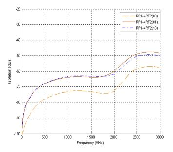
Figure 5. RF1 to RF2 Isolation
