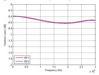
Figure 5. Insertion Loss vs. Temp (RFC-RFX)
