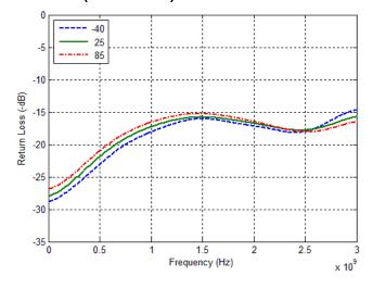
Figure 14. Active Port Return Loss vs. V<sub>DD</sub> (RF2 Active)
