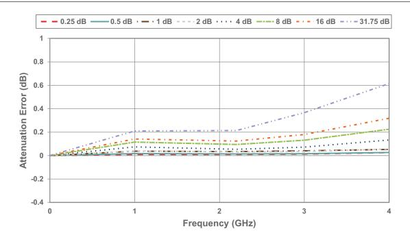
Figure 22 • 0.25 dB Attenuation Error vs Frequency
