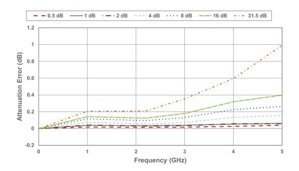
Figure 26 • 0.5 dB Attenuation Error vs Frequency
