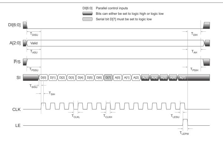
Figure 4 - Latched Parallel/Direct Parallel Timing Diagram
