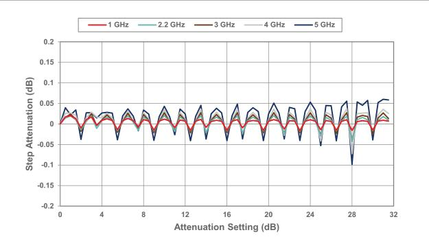
Note: \* Monotonicity is held so long as step attenuation does not cross below -0.5 dB.
