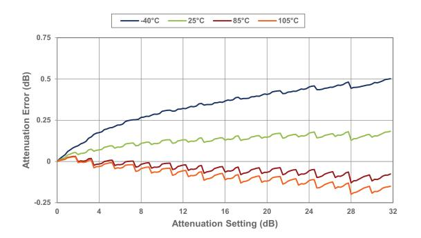
Figure 16 • Attenuation Error @ 3000 MHz vs Temperature
