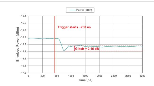
Figure 31 • Attenuation Transient (15.75–16 dB), Typical Switching Time = 275 ns
