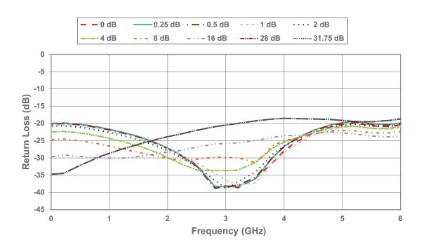
Figure 8 - Output Return Loss vs Attenuation Setting
