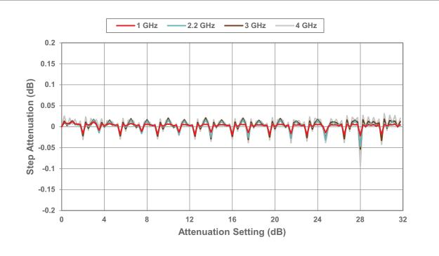
Note: \* Monotonicity is held so long as step attenuation does not cross below -0.25 dB.
