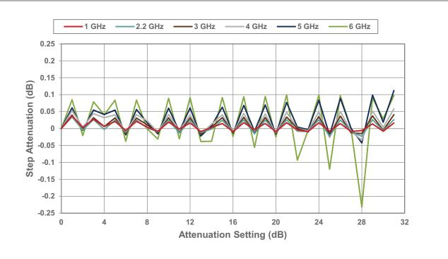
Note: \* Monotonicity is held so long as step attenuation does not cross below -1 dB.
