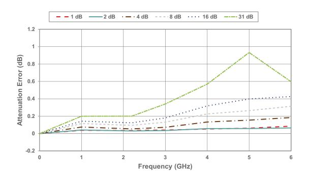
Figure 30 • 1 dB Attenuation Error vs Frequency
