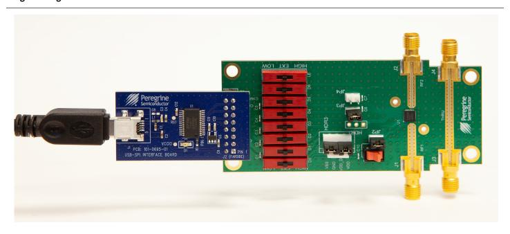
Figure 14 • PE43650 USB Interface Board Connected to the Evaluation Board for Latched Parallel and Serial Programming—Side View
