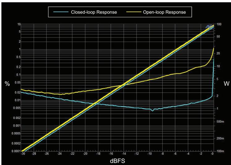
Switching frequency 404 kHz, +/-20V power supplies, 8 Ohms, open loop, timing = 0s: THD vs Level @ 1 KHz - SPDIF input
