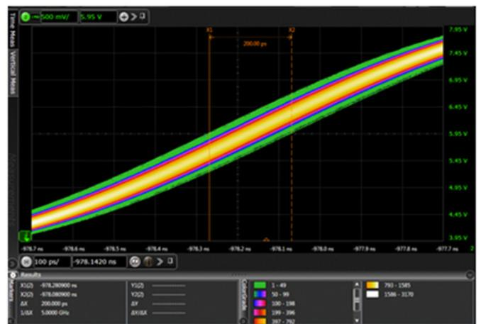
The jitter range for a GaN FET switched by the PE29102 is impressively narrow, with a low standard deviation figure.
