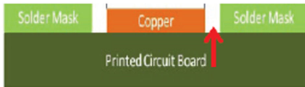
Figure 13. NSMD Pads (Solder Mask away from Copper)
