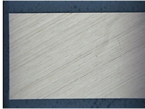
Figure 3. WLCSP Back Side with Opaque Finish
